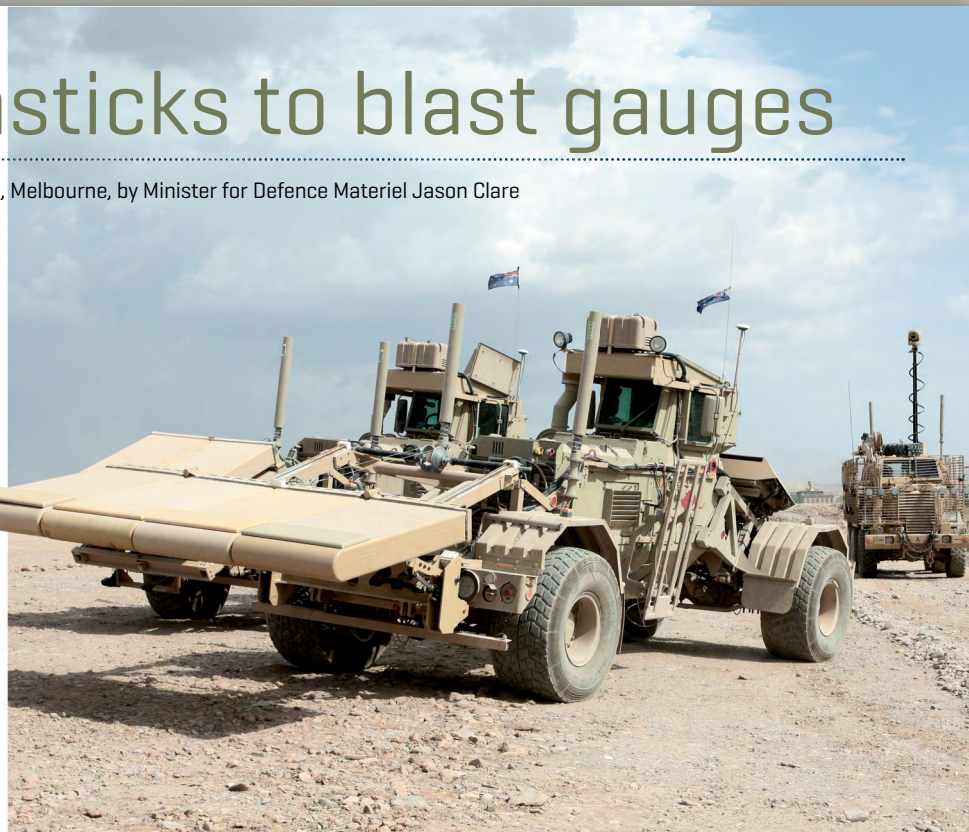
Two Huskey mine detection vehicles with ground-penetrating radar arrays out front, followed by a Buffalo, which Australian engineers are using in Afghanistan to detect and deal with IEDs. Pic Brian Hartigan.
