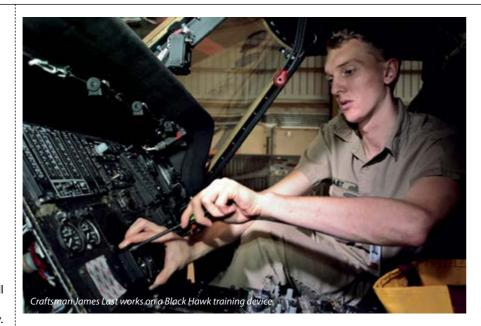
SAMT IS A TERRIFIC TRAINING SIMULATOR THAT ALLOWS STUDENTS TO VIRTUALLY **REMOVE COMPONENTS FROM AN AIRCRAFT, USING CORRECT TOOLS TO TEST OR REPAIR** THE COMPONENT BEFORE REPLACING IT
