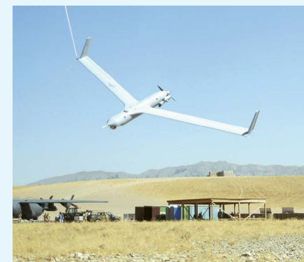
ScanEagle was originally designed to operate from ships – hence, it is launched by catapult and recovered by cherry picker and bungee cord.
