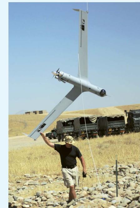
ScanEagle was originally designed to operate from ships – hence, it is launched by catapult and recovered by cherry picker and bungee cord.
