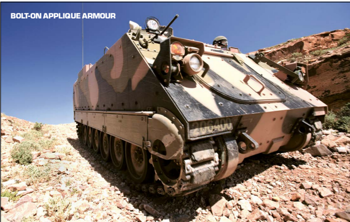
M113AS4 ALV HAS A STRETCHED HULL, SIXTH ROAD WHEEL AND A 6 TONNE PAYLOAD
