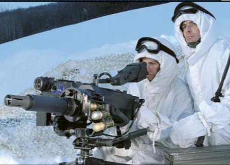
GENERAL DYNAMICS' MK 47 MOD 0 STRIKER IS A LIGHTWEIGHT 40MM AGL WITH ADVANCED FIRE-CONTROL SYSTEM. PIC GD&P
