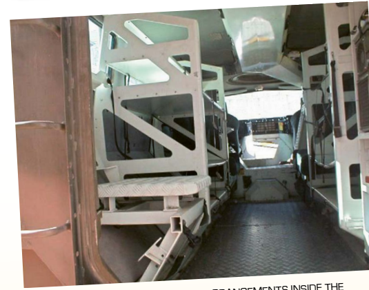
AN INTERNAL VIEW OF THE RACKING ARRANGEMENTS INSIDE THE DIRECT FIRE WEAPONS VEHICLE.
