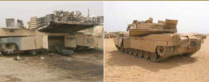
LEFT: MOST LOSSES WERE ATTRIBUTED TO MECHANICAL BREAKDOWN OR EXTERNAL STOWAGE FIRES. THE VEHICLES WERE STRIPPED BEFORE BEING ABANDONED. RIGHT: AFTER SURVIVING TWO RPG STRIKES THIS M1 WAS STOPPED BY 25MM HITS TO THE REAR ENGINE COMPARTMENT.
