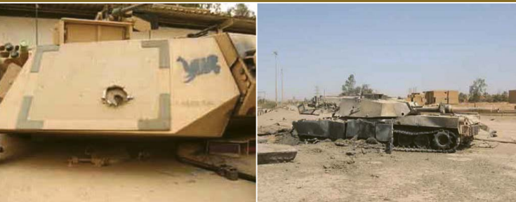
LEFT: FRONTAL TURRET AND HULL ARMOUR CONTINUES TO PROVIDE EXCELLENT CREW PROTECTION AS SHOWN WITH THIS 25MM STRIKE. RIGHT: AFTER A BREAKDOWN IT TOOK A GRENADE, A SABOT ROUND AND TWO MAVERICK MISSILES TO DESTROY THIS M1 TO PROTECT ITS SECRET TECHNOLOGY.
