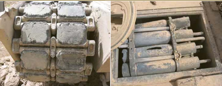
LEFT: ROADWHEELS AND TRACKPAD WEAR PROVED TO BE SIGNIFICANT OVER THE LONG DISTANCES TRAVELLED. A HIGH RATE OF FAILURE FOR ROAD ARMS (THREE). RIGHT: EVEN AFTER BEING HIT, AMMUNITION BLAST DOORS PROTECTED CREW AS DESIGNED, WITH THE CREW SURVIVING.
