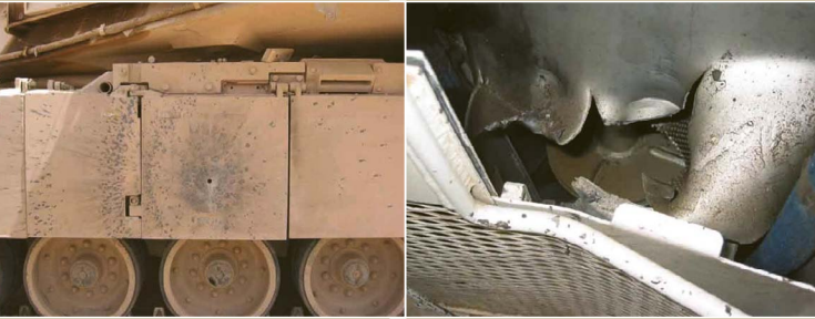
LEFT: ANTI-ARMOUR RPG ATTACK TO LEFT SIDE. NON-BALLISTIC SKIRTS REPEATEDLY PENETRATED BY ANTI-ARMOUR RPG FIRE. ANTI-PERSONNEL RPG ROUNDS CAUSED ONLY COSMETIC DAMAGE. RIGHT: RPG PENETRATION INTO HYDRAULIC RESERVOIR.
