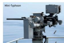
The system has a high level of accuracy, weighs 170kg and can be installed without structural penetration of a ship's deck.
