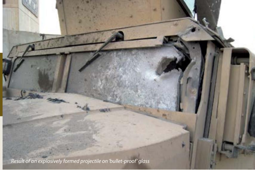
Result of an explosively formed projectile on 'bullet-proof' glass
