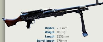
The Belgian-made general support machine gun (GSMG) FN MAG58 is designed in the 1950s for general support purposes.
