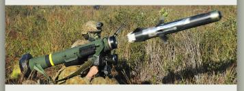
Missile weight 11.8kg Warhead weight 8.4kg Missile length 110cm Flight time 7sec per 1000m
