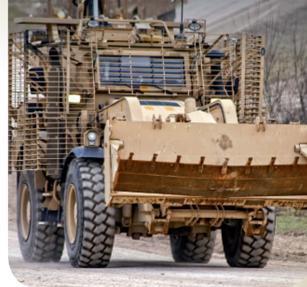
UK Talisman theatre-entry standard (TES) High Mobility Engineer Excavator (HMEE) with upgraded armour kit, to include underbelly blast plate, armour cab protection, rocket screen bar armour, blast attenuating seat, roof escape hatch and improved situational awareness thermal imagery camera suite. The pictured HMEE is conducting a route-proofing and clearance mission with UK forces in Afghanistan and will soon be doing the same for Australian forces.
